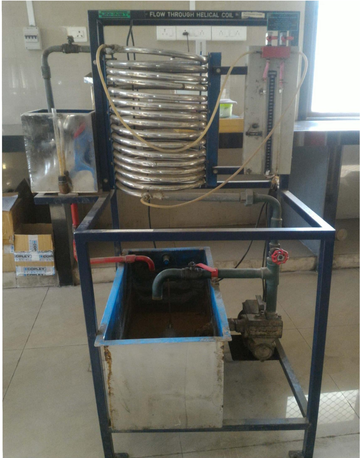
Set up 3: Flow Through Helical Coil
